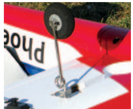
The wings are designed for retracts.
