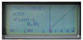
It's important that the throttle curve is linear to start the calibration process. It can be changed to your normal curve after the calibration is complete.
