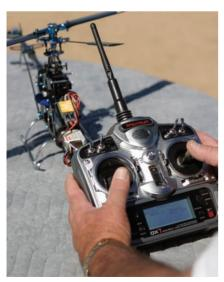
Don't forget to remove the pinion gear or move the motor away from the maingear since you will need to start and stop the motor during the calibration process.
