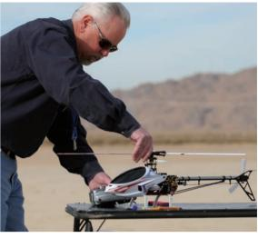
easy on initial spool up of the blades on the ground. If you do any float flying on water, soft start is a big advantage since it significantly limits the torque effect as the helicopter spools up.
