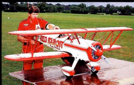
Sixth in Team: Jim Sandquist (shown here) and Jess Larson; 1/4-scale Super Stearman; 45 lb.; 96" span; Bob Dively kit; balsa, ply, fiberglass, aluminum; Sig Koverall and Randolph dope; Bob Smith glue and Pica aliphatic resin; hand-painted markings; Brison/Sachs 4.2 gas; Clark 22x12; Futaba, 5 channels; 6 servos; Robart, fixed, shock-absorbing Oleo struts; Bennett smoke system; FTE dummy engine.
