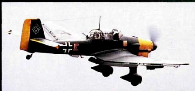
Seventeenth in Expert: Jim Wilkinson; 1/8-scale JU-87B Stuka; 21 lb.; 91" span; wood, fiberglass cowl and pants; acrylic enamel, Zap; airbrushed markings; Zenoah G-38 gas; Zinger 18x6/10; Futaba
