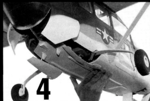
Here's Ramon's drive mechanism for his Cessna landing gear. The electric drive motor is controlled with microswitches, and universal joints drive and lock the gear up and down. The entire unit is mounted on a removable aluminum plate.
