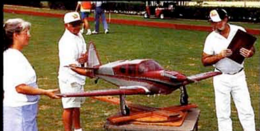
Seventh in Expert: Corvin Miller; 1/4-scale Globe Swift; 21 lb.; 80" span; scratch-built; balsa and ply; Imron (same as full-size); Z-Poxy; hand-painted markings; O.S. 1.60 twin; Zinger 16x6/10; Pro Power; Airtronics Infinity 6-channel; 10 servos; scratch-built retracts; Vailly Aviation wheels; Robart tires.
