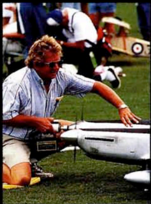
Above—twenty-fifth in Expert: Art Johnson; 1/8-scale North American P-82; 31 lb.; 102.5" span; all scratch; balsa, ply, aluminum tape finish; Zap; hand-painted markings; 2 O.S. 1.08 engines; Zinger 16x6; Byron sport fuel; Futaba 9 AUP; 18 servos; scratch retracts;
