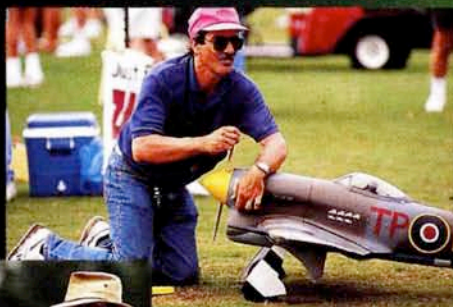
Left—twenty-first in Expert: Bob Underwood; 1/4.5-scale Hiperbipe home-built; 15 1/4 lb.; 73" span; all scratch; balsa, plywood; built-up wings; Coverite with Du Pont automotive enamel; Zap and aliphatic resin; painted markings; O.S. 1.60 twin cylinder; Zinger 18x6/10; Cool Power; Airtronics Vision, 4 channels; 5 servos; Du-Bro air-
