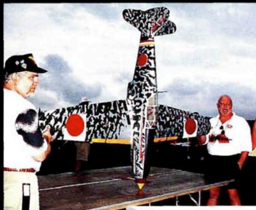
Right: first in Team: Bob Violett (right) and Jerry Caudle; 1/6.5-scale P-80 Shooting Star; 16 lb.; 80" span; BVM kit; foam; balsa and fiberglass; Coverite Presto with PPG acrylic paint; Zap; Dry-Set markings; BVM .91; Viojett fan unit; JP-4 fuel; JR, 10 channels; 12 servos; BVM retracts and wheels; lights; sliding canopy and split flaps; wheel brakes; speed brakes; tank drop.
