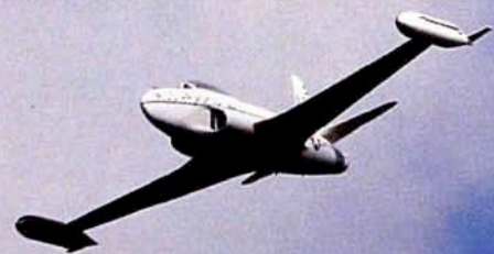
Second in Expert: Garland Hamilton; 1/6.5-scale F-80 Shooting Star; 18 lb.; 80" span; BVM kit; foam/fiberglass; BVM .91S; BVM Viojett fan unit; BVM special fuel; Airtronics Infinity; BVM retracts; second—'94 Top Gun Expert.
