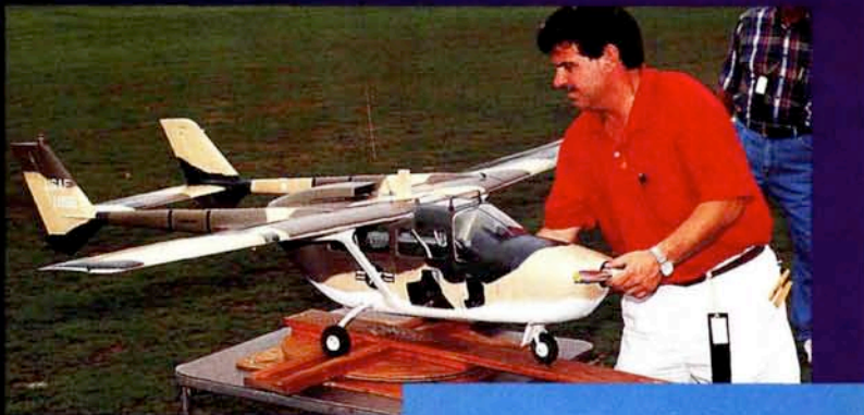
Above & right—third in Expert: Ramon Torres; 1/6-scale Cessna O-2A; 18.5 lb.; 91" span; all scratch; fiberglass and molded honeycomb composite; Zap; HobbyPox paint with K&B hardener; hand-painted markings; two O.S. .46 engines with 12x6 Rev-Up props; Texxon fuel; Futaba 9 PCM; 13 servos; scratch-built, geared electric retracts with sequencing gear doors; fifth—FAI '92 World Championships.
