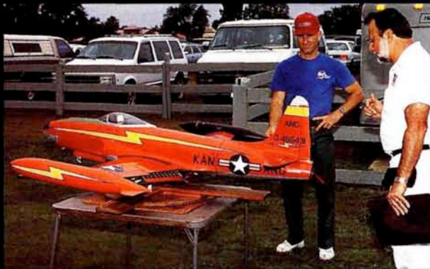
Second in Expert: Garland Hamilton; 1/6.5-scale F-80 Shooting Star; 18 lb.; 80" span; BVM kit; foam/fiberglass; BVM .91S; BVM Viojett fan unit; BVM special fuel; Airtronics Infinity; BVM retracts; second—'94 Top Gun Expert.
