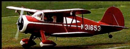
Ninth in Expert: Charlie Nelson; 2.8"/ft.-scale Waco VKS7F; 32 lb.; 93" span; balsa, ply, fiberglass and aluminum; dope over Sig Koverall; Zap; Hand-painted markings; Seidel 7-cylinder radial; Zinger 22x10; Red Max; Airtronics Vision, 8 channels; 9 servos; flaps and retractable, wing-mounted landing lights; model was built around the dimensions of the Seidel engine.
