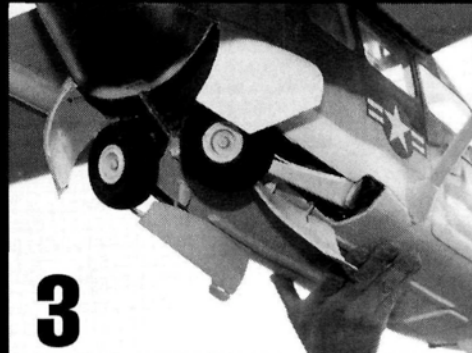
Ramon Torres' Cessna 0-2A has a rearward-retracting main landing gear with sequencing landing-gear doors. This fascinating, functional design looks deceptively simple.
