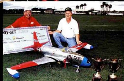
Right: first in Team: Bob Violett (right) and Jerry Caudle; 1/6.5-scale P-80 Shooting Star; 16 lb.; 80" span; BVM kit; foam; balsa and fiberglass; Coverite Presto with PPG acrylic paint; Zap; Dry-Set markings; BVM .91; Viojett fan unit; JP-4 fuel; JR, 10 channels; 12 servos; BVM retracts and wheels; lights; sliding canopy and split flaps; wheel brakes; speed brakes; tank drop.
