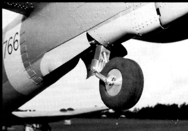
Sepp also duplicated the complicated, intricate tail-wheel retract mechanism and its landing-gear-door linkage—no small task!
