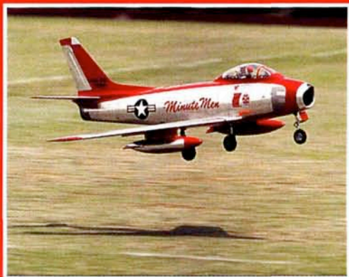
First in Expert: Terry Nitsch; 1/8-scale F-86 Sabre Jet; 14 lb.; 58" span; BVM kit; foam/fiberglass; Zap CA and Z-Poxy; Coverite Presto metal finish with Ditzler acrylic enamel paint; BVM .91; Viojett fan unit; Powermaster JP-4 fuel; JR PCM 10SX; 9 channels with 13 servos; BVM retracts and tires with Glennis wheels; winner—'94 Top Gun and '94 Scale Masters.
