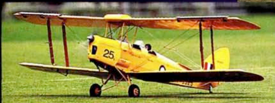
Eighth in Expert: Mike Barbee; 1/4-scale deHavilland 82 Tiger Moth; 16 lb.; 88" span; Duncan Hutson plans; balsa, spruce and ply; Delron base and clearcoat urethane over Supershrink Coverite; Zap; Dry-Set markings; Laser 150; APC 16x8; Cool Power; Futaba 1024 ZAP; 5 channels; 6 servos; operating LE slats; cable control system; Best Civilian—'94 Top Gun.
