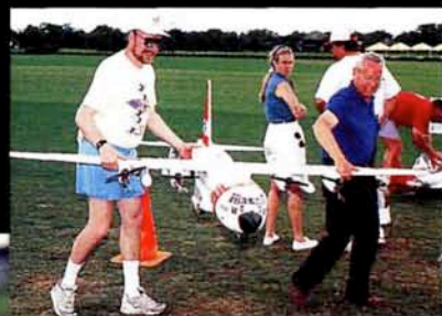
Thirty-second in Expert: Skip Mast (right); 1/16-scale Lockheed HC-130H; 17 lb.; 97" span; scratch-built from own plans; balsa-covered foam; epoxy finishing resin, lacquer primer, epoxy paint; Zap; 4 K&B .21 engines; Master Airscrew 9x4; Airtronics; 7 servos; Zinger wheels; flaps; scratch-built retracts; strobe light; operating cargo door with cargo drop. Rivets and panel lines made with latex paint applied with old drafting pen.
