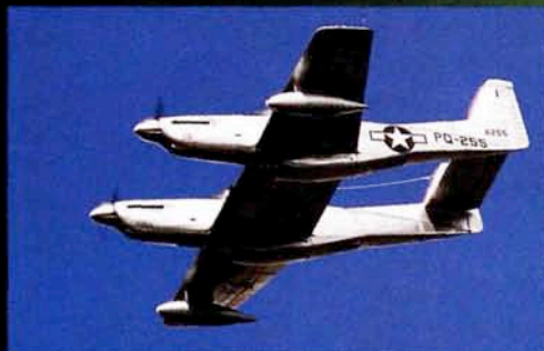
Above—twenty-fifth in Expert: Art Johnson; 1/8-scale North American P-82; 31 lb.; 102.5" span; all scratch; balsa, ply, aluminum tape finish; Zap; hand-painted markings; 2 O.S. 1.08 engines; Zinger 16x6; Byron sport fuel; Futaba 9 AUP; 18 servos; scratch retracts;
