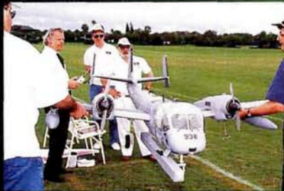
Left—twenty-first in Expert: Bob Underwood; 1/4.5-scale Hiperbipe home-built; 15 1/4 lb.; 73" span; all scratch; balsa, plywood; built-up wings; Coverite with Du Pont automotive enamel; Zap and aliphatic resin; painted markings; O.S. 1.60 twin cylinder; Zinger 18x6/10; Cool Power; Airtronics Vision, 4 channels; 5 servos; Du-Bro air-
