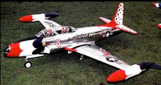
Fifth in Team: Steve Elias and Ian Richardson; 16.5-scale T-33 Thunderbird; 16.5 lb.; 80" span; BVM kit; fiberglass; foam and wood sheeting; Coverite Presto; epoxy paint; Zap; Dry-Set markings; BVM .91; Viojett fan unit; JP-4 fuel; Futaba 9ZAP; 10 servos; split flaps; BVM retracts; tires and brakes.
