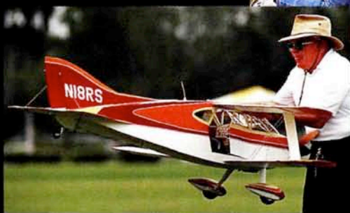
Left—twenty-first in Expert: Bob Underwood; 1/4.5-scale Hiperbipe home-built; 15 1/4 lb.; 73" span; all scratch; balsa, plywood; built-up wings; Coverite with Du Pont automotive enamel; Zap and aliphatic resin; painted markings; O.S. 1.60 twin cylinder; Zinger 18x6/10; Cool Power; Airtronics Vision, 4 channels; 5 servos; Du-Bro air-
