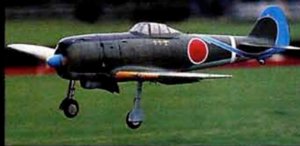
Thirty-fourth in Expert: Wayne Siewert; 1/6-scale KI-84 Frank; 32 lb.; 88" span; Aero Tech kit; carbon-fiber fuse; foam and balsa aluminum wing spar; acrylic lacquer automotive paint; industrial epoxy; hand-painted markings; Zenoah G-62; Zinger 20x8/14; Futaba; 7 servos; Century Jet retracts with Yellow Aircraft wheels; kit derived from Don Smith Plans; fully detailed aluminum cockpit.
