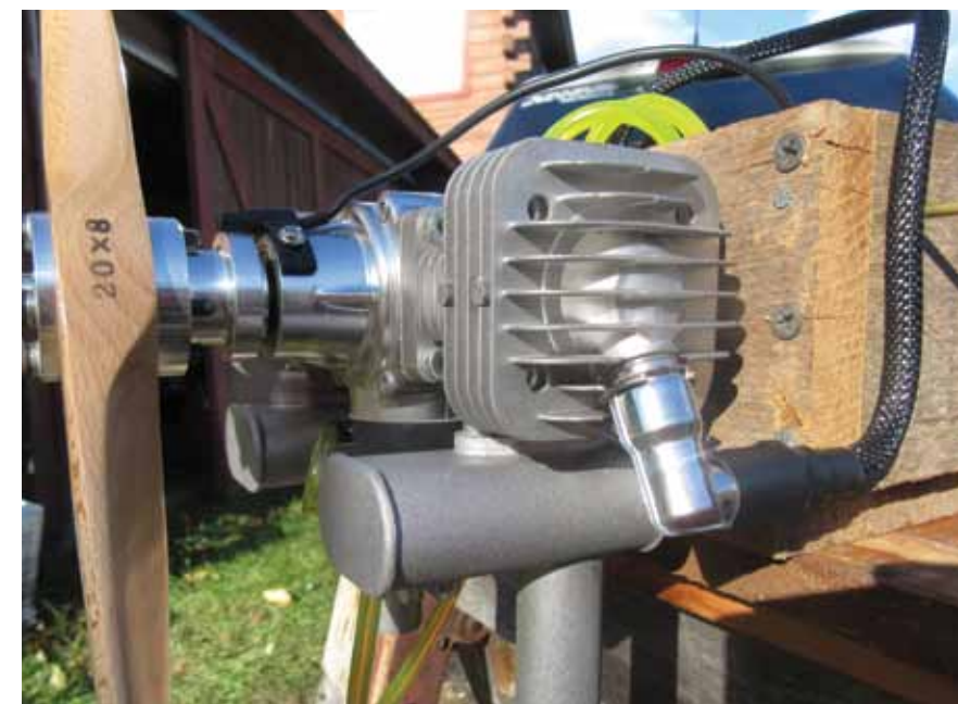
As you can see, the spark plugs are installed at a downward angle making the engine narrower.
