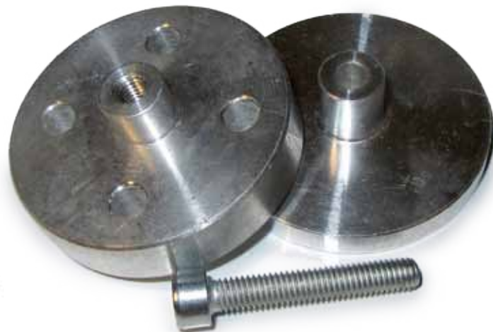
To properly drill the propeller-attachment boltholes, RCGF USA includes a drilling jig that makes the task quick and accurate.
